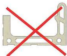
Channel piece with cavities: The result is risks with regard to hygiene, stability and frost resistance (not produced by AGROB BUCHTAL)
