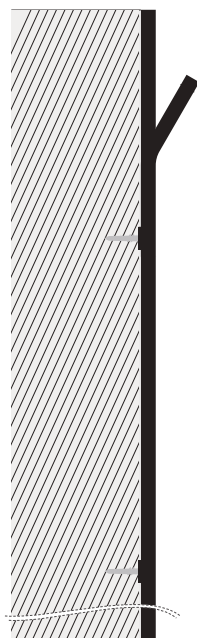
Fixing brackets from the top (100 - 835 - 830 - 835 - 100) (mm)
